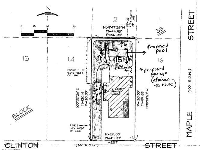
1.) THE RATIO OF CLOSURE OF UNADJUSTED FIELD OBSERVATIONS IS NOT GREATER THAN I PART IN 5,000.
